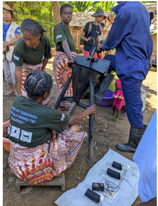
Photo: Local community biocharcoal production in Nosy Fala, Madagascar. Source: NIRAS evaluation team
